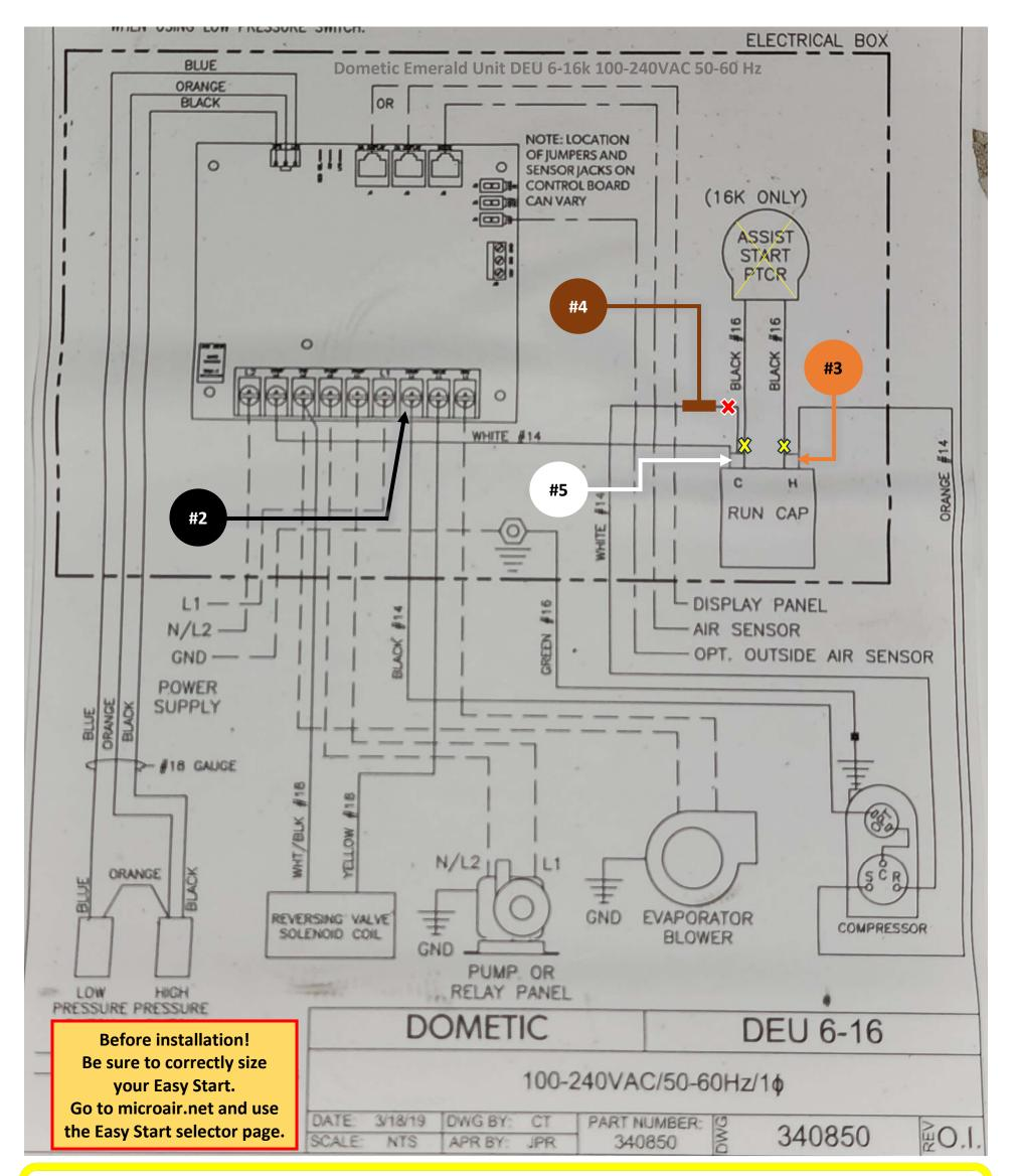
1. Before Easy Start installation! All connectors used must be 600VAC rated!
