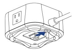
4. Thread the mounting nut onto the mounting bolt
