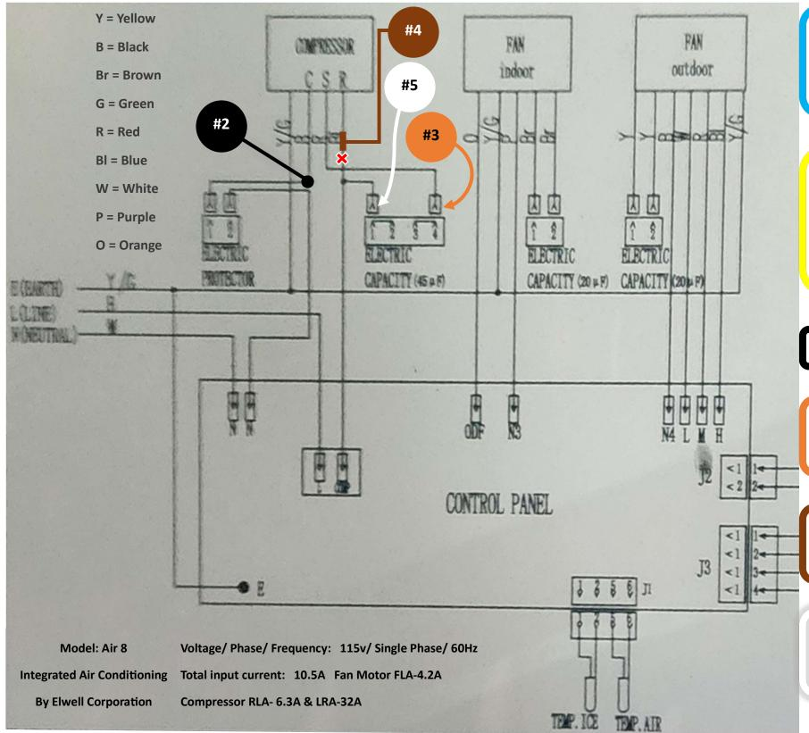
On your wiring diagram the compressor will have C, S and R. On the compressor CSR will be on the cover over these wires.
