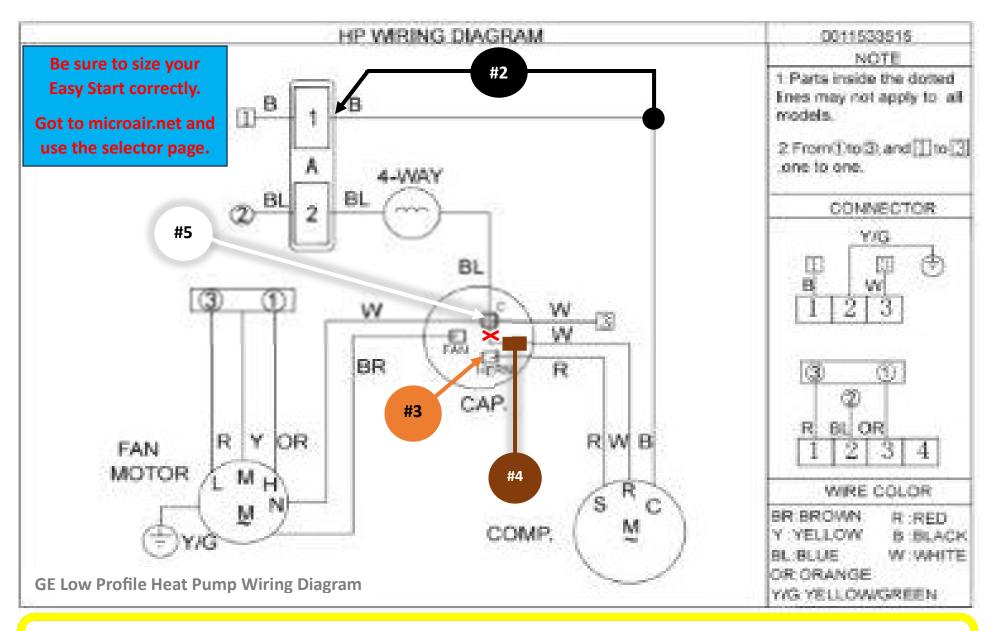
1. Before Easy Start installation! All connectors used must be 600VAC rated.
